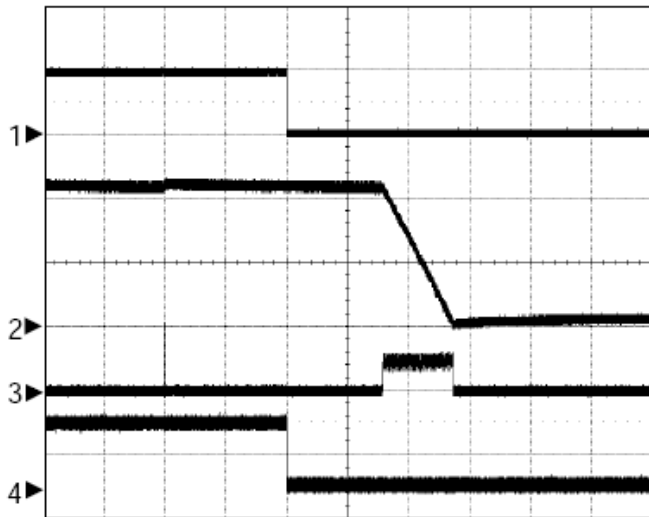
Shutdown with Soft-Stop at No Load
