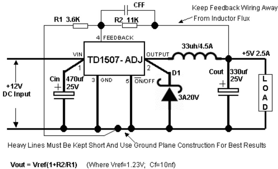
Figure 12. Typical Application of TD1507 For ADJ
