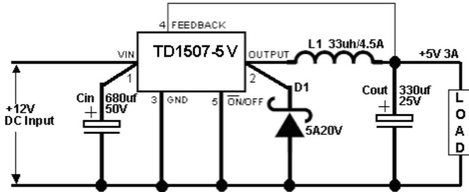
Figure 11. Typical Application of TD1507 For 5V
