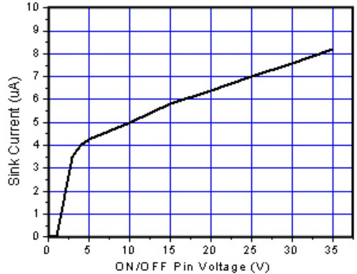
Figure 9. ON/OFF Pin Sink Current
