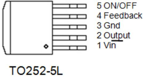
Figure 2 Pin Configuration of TD1507 (Top View)
